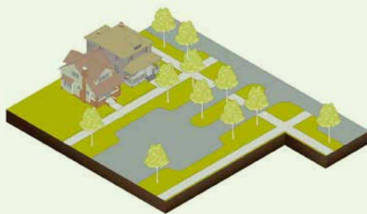
Gateway entrance with median and curb extensions
